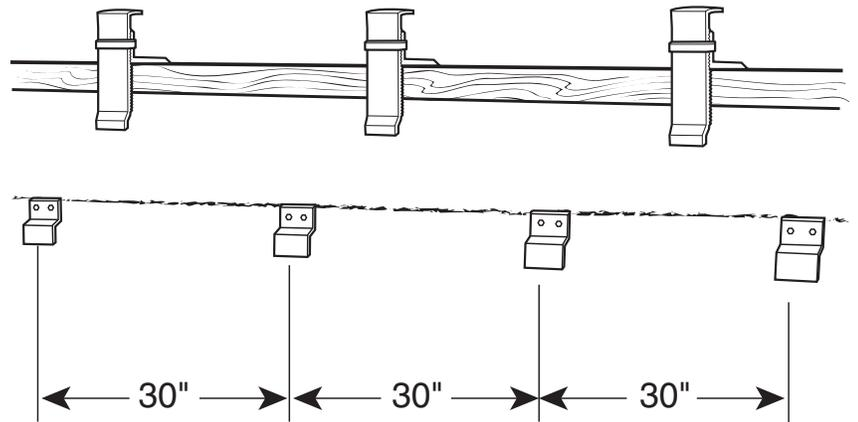
**3.** Once Clips are installed, lock Fascia Extender to bottom of Extender Clips and slide Fascia Extender under Fascia Holder and fasten.
